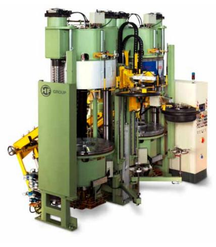
Nitrogen-operated, hydraulic tire press (courtesy of Harburg-Freudenberger Maschinenbau GmbH)
